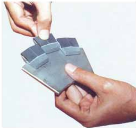
Super-D-Canter scroll showing the tungsten carbide tiles in position.
