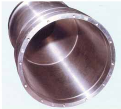
Stainless steel centrifuge bowl after 7 years of continuous operation.
