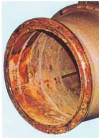
Carbon steel centrifuge bowl after 1 year of operation.
